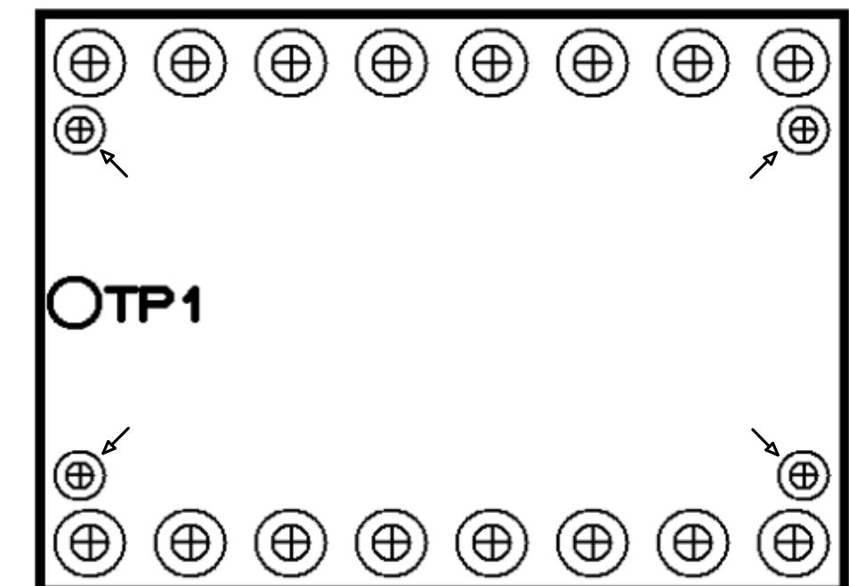
Backside is copper plane: Corner pads and TP1 tied to plane.
