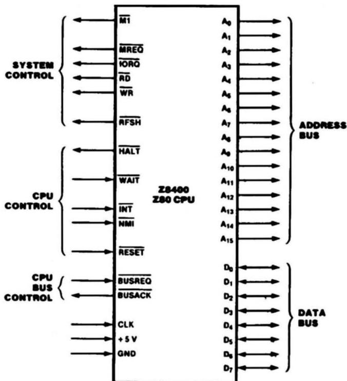
Figure 1. Pin Functions
