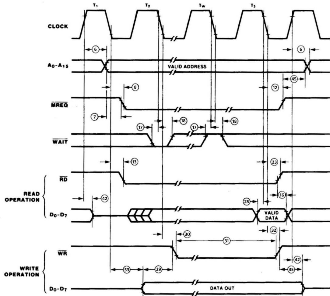
Figure 6. Memory Read or Write Cycles
