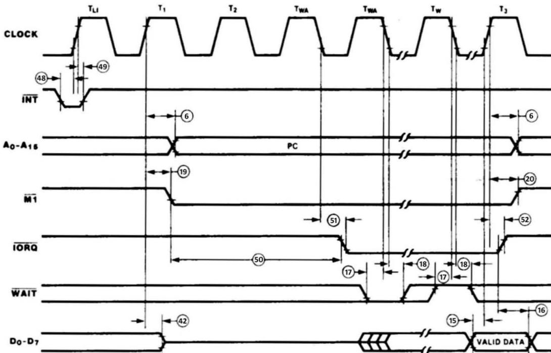
**Non-Maskable Interrupt Request Cycle.** NMI is sampled at the same time as the maskable interrupt input INT but has higher priority and cannot be disabled under software control. The subsequent timing is similar to that of a normal
