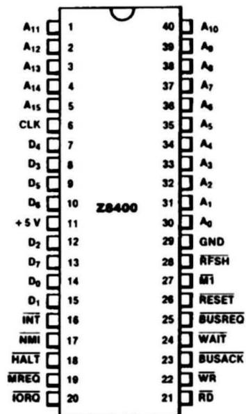
Figure 2. 40-pin Dual-In-Line (DIP), Pin Assignments
