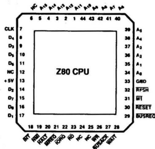
Figure 2b. 44-Pin Chip Carrier Pin
