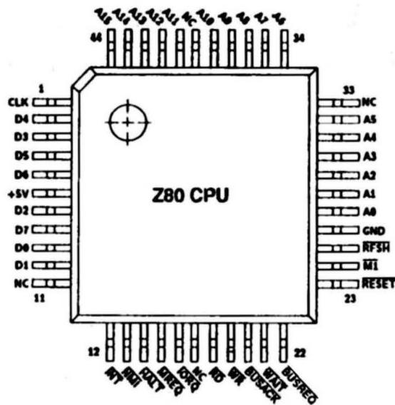
Figure 2a. 44-Pin LQFP, Pin Assignments
