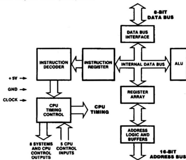
Figure 3. Z80C CPU Block Diagram
