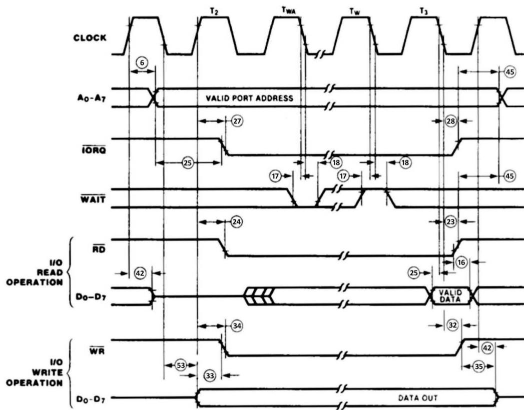
$T_{WA}$  = One wait cycle automatically inserted by CPU.
