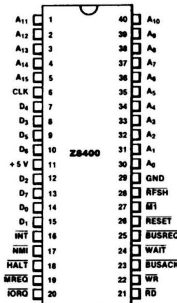
Figure 2. 40-pin Dual-In-Line (DIP), Pin Assignments
